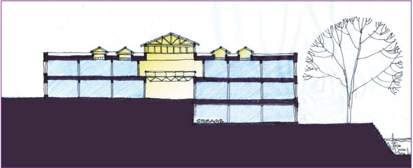
A section through the Beaumont Mill illustrating the introduction of a clerestory and common atrium for residential uses
