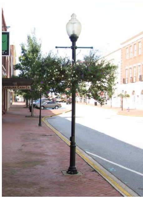
The standard, and problematic, acorn light fixture casts very poor light in an urban setting
